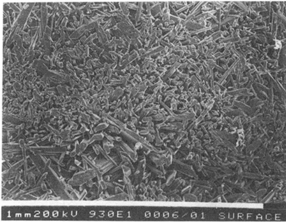
Fig. 6 Crystals formed on the plate surface at a flow velocity of 21.9 cm/s
